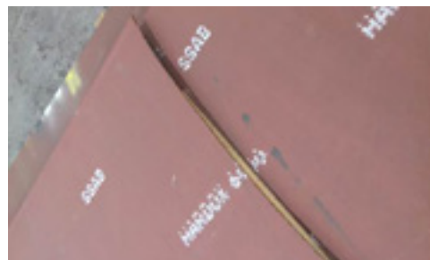
Example of a three-point force during storage.
